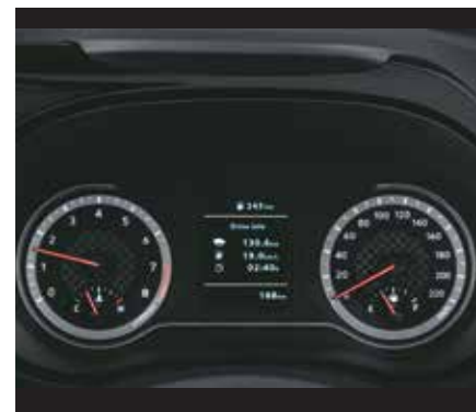
8.89 cm (3.5") Speedometer with multi information display
