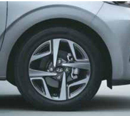
R15 (D = 380.2 mm) Diamond cut alloy wheels
